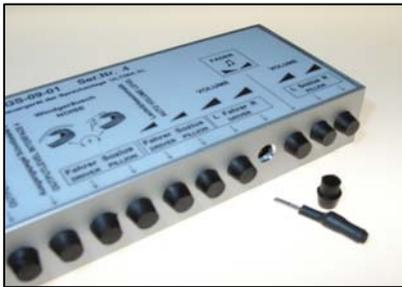
On one side of the control device there are 13 black rubber plugs to avoid water entering the system.
