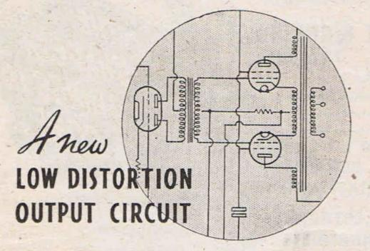
The new low distortion output circuit (an Acoustical Provisional Patent) incorporated in the M31 Amplifier provides a very high standard of reproduction-The output valves operate partly as triodes with cathode follower output and partly as tetrodes with negative feedback, thus giving considerable cancellation of generated harmonics and a high damping factor. Just one reason why you prefer Acoustical.
